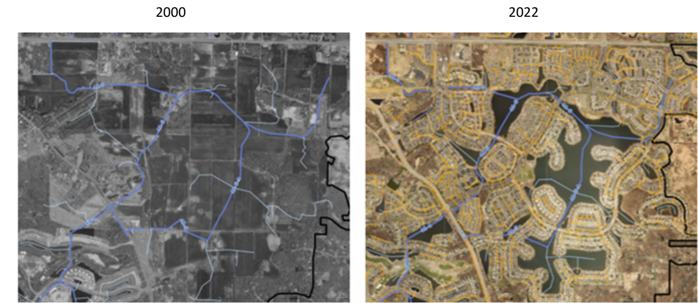
Figure 3. Location of Sunrise Lake before (2000) and after (2022) its creation as a man-made lake. The legal flow path of the Anoka County Ditch 41 system was maintained.
