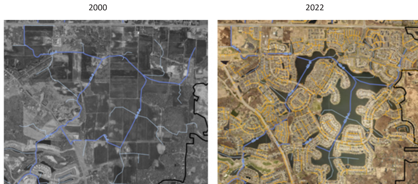
Figure 3. Location of Sunrise Lake before (2000) and after (2022) its creation as a man-made lake. The legal flow path of the Anoka County Ditch 41 system was maintained.
