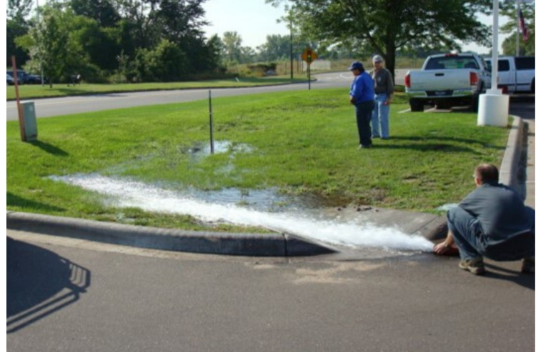
Testing an infiltration basin
