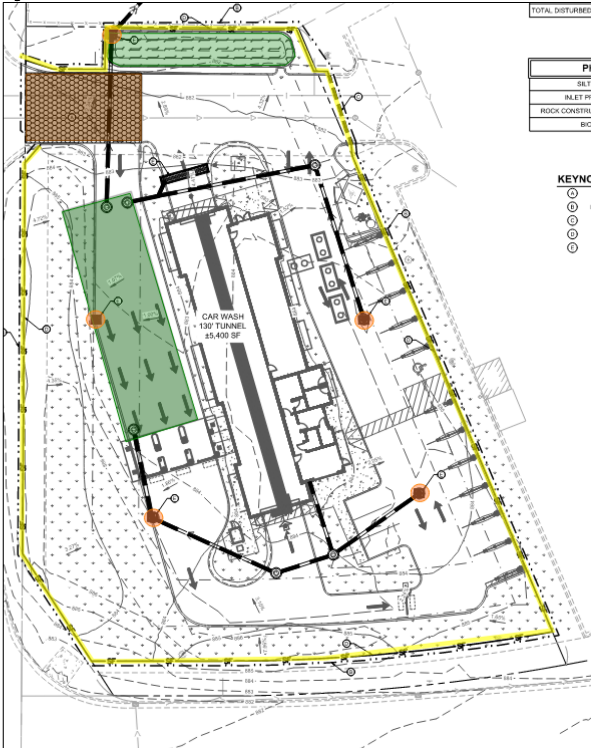
Figure 2. Erosion and Sediment Control Plan
