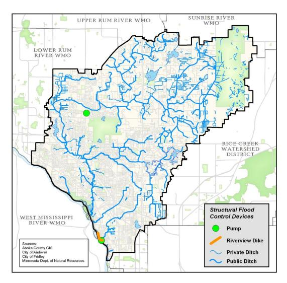
**Channel Alteration** Approximately 285 miles of stream channel have been straightened, deepened and in some cases widened for the sole purpose of moving water to facilitate drainage and discourage flooding.
