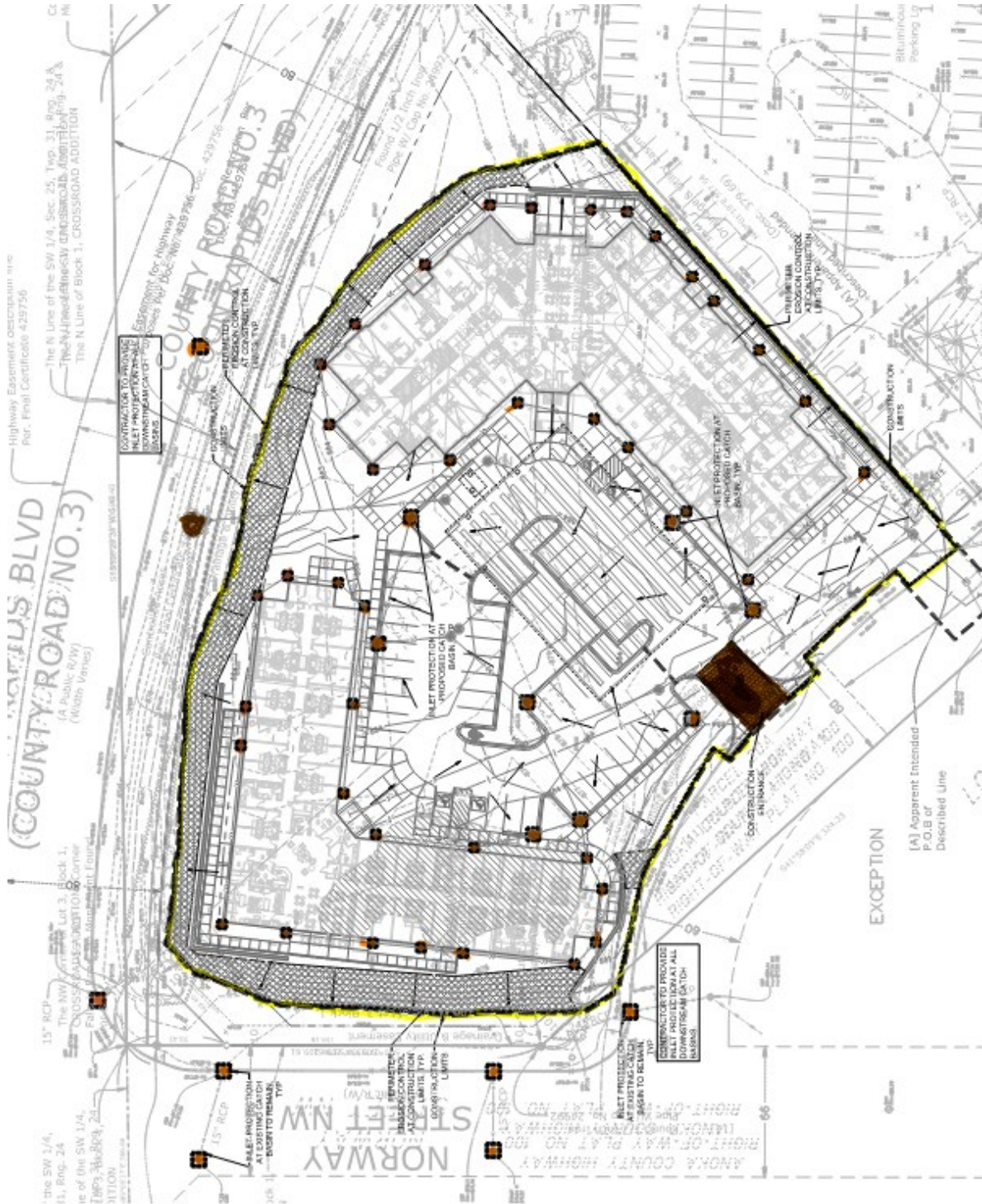
Figure 2: Erosion & Sediment Control Plan
